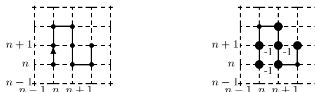
Figure 1.3. The folding f on \mathbb{Z}^2 lattice (left). Contacts and energy contributions of the string HHPHHPH w.r.t. the same folding (right).
